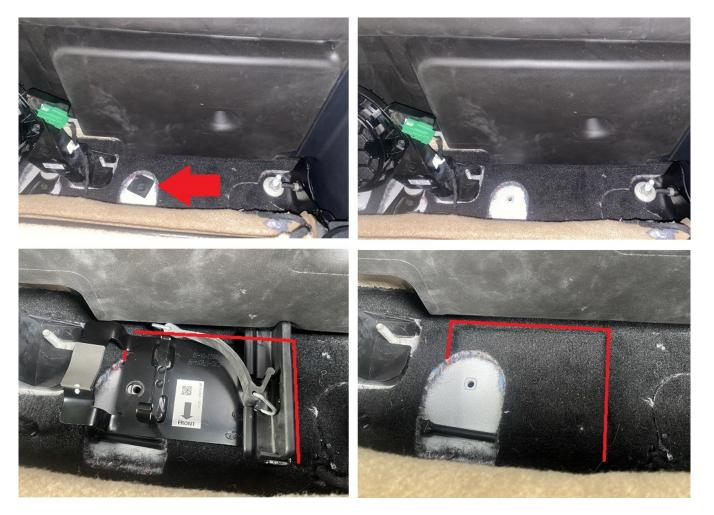
Using a razor blade cut along the marked line be sure to keep clear of any wires under the carpet. Attach the front of the bottle jack using the provided M8 bolt. Using the provided self-tapping bolt, attach the rear of the bottle jack mounting plate to the cab of the truck, **Note:** you are threading into aluminum, it is best to get it started with a drill and finish the last few turns by hand.
