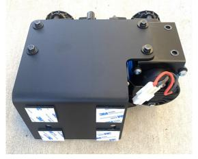
Using a 13mm wrench, install the compressor using the bolts removed in step #1. When installing this bracket push it as far back as possible to prevent the compressor from coming in contact with the seat when in the folded-up position. Attach the push to connect "T" air line fitting into the compressor using a 14mm wrench. Screw on the two ARB air filter screens as below.
