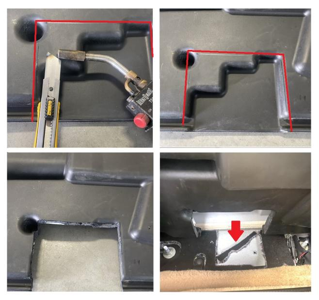
Reinstall the rubber pad, the (3) plastic push in clips, then reattach the rear speaker. Using a razor blade cut off the small carpet piece as shown in the 4<sup>th</sup> photo above.
