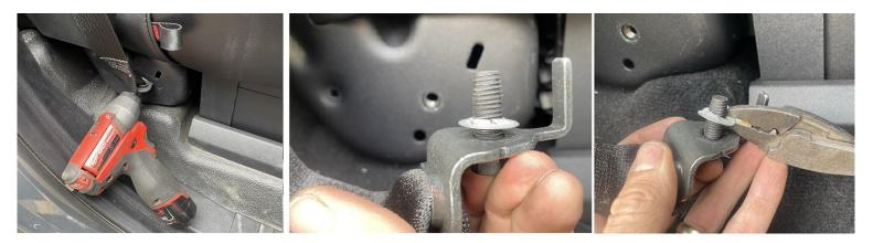
Install the air chuck mounting bracket. These brackets are symmetrical and will work on either side of the vehicle. Reinstall the seat belt mounting bolt as shown below then install the  $\frac{1}{4}$ " diameter self-tapping screw using a  $\frac{3}{8}$ " open-end wrench. Thread the push to connect fitting into the air chuck using a  $\frac{9}{16}$ " &  $\frac{13}{16}$ " wrench. Firmly tighten this connection. Repeat this procedure to the opposing side of the vehicle.
