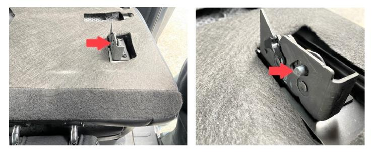
Connect the ¼" diameter, 60" long airline to the push to connect fitting on the driver side, the opposite end will connect to the "T" push to connect airline fitting on the ARB compressor. Carefully route the air line under the carpet where possible as outlined in red to reduce any potential rattling or damage.
