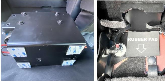
Attach the jack to the mounting plate using the provided (4) Velcro straps. (1) 8" strap around the jack handle pump, to reduce rattles, (2) 12" Velcro straps attaching the jack to the mounting plate, and (1) 12" Velcro strap attaching the handle to the jack.
