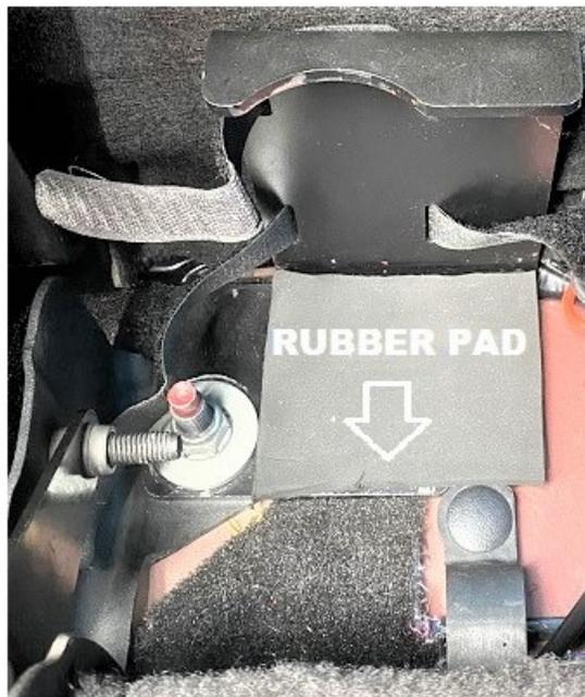
Attach the jack to the mounting plate using the provided (4) Velcro straps. (1) 8" strap around the jack handle pump, to reduce rattles, (2) 12" Velcro straps attaching the jack to the mounting plate, and (1) 12" Velcro strap attaching the handle to the jack.
